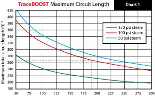
Temperature difference (heating medium temperature - process temperature) (°F) \* Maximum circuit length includes: supply, tracing, and return.
