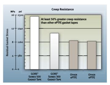
Creep resistance data based on EN13555 using 15mm x 3mm tape formed into a 150mm skived ring.  $P_{\rm QR}$  values were obtained at 30 MPa initial gasket stress at 150°C.
